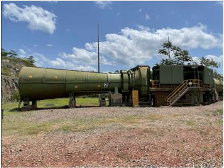
Figure 18-22: Howden Primary Ventilation Fans, Paboase Underground Mine
