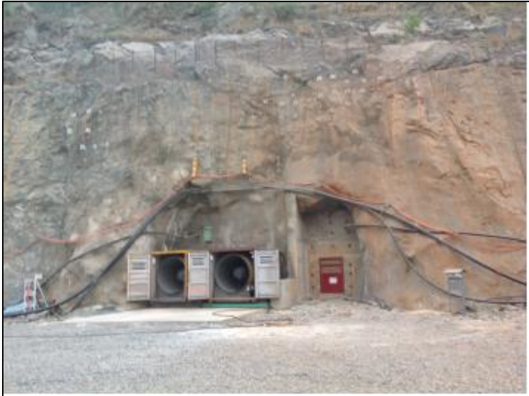
Figure 18-23: Swedvent Primary Ventilation Fans, Akoti Underground Mine
